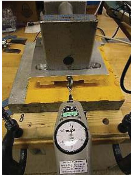
Photo No. 25 Typical FM 3-C1028 Test Detail
