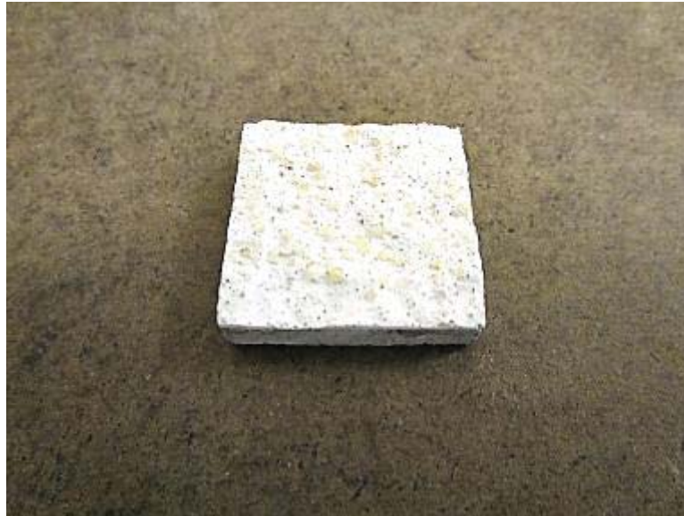
Photo No. 15 Typical Smoke Density Specimen Detail
