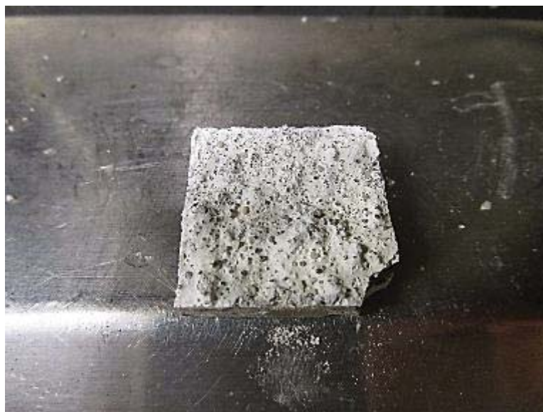
Photo No. 18 Typical Smoke Density Specimen Detail
