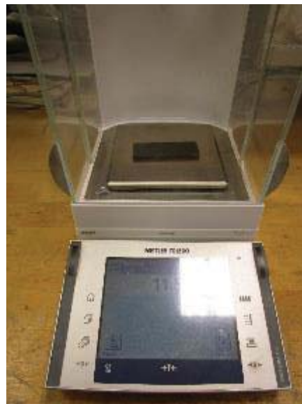
Photo No. 24 Water Absorption Test In-Progress Detail
