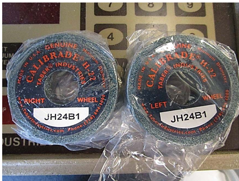
Photo No. 14 H-22 Calibrade Abrasion Wheel Detail
