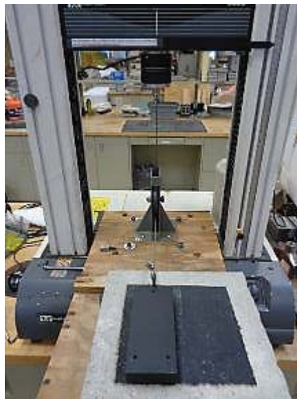
Photo No. 26 Typical ASTM F609 Test Setup Detail
