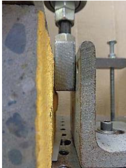
Photo No. 9 Bond Strength Test Setup Detail
