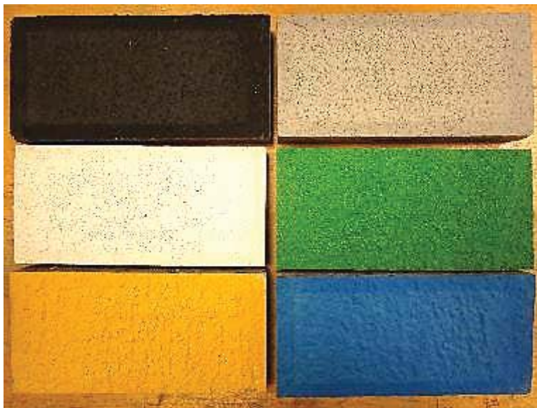
Photo No. 6 Post-Weathering Specimen Detail
