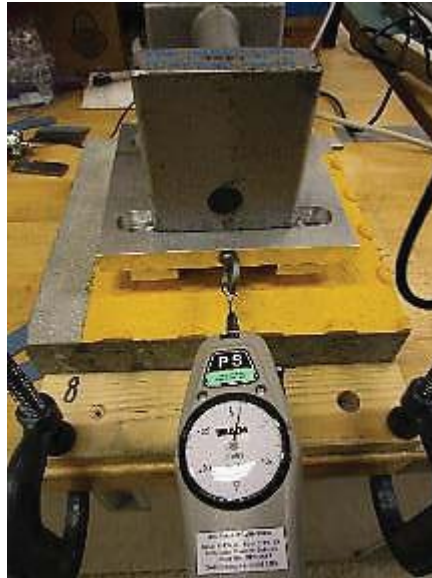
Photo No. 25 Typical FM 3-C1028 Test Detail
