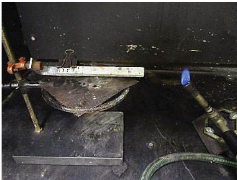
Photo No. 20 Typical Rate of Burn Test Setup Detail
