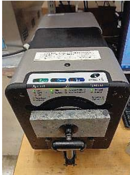
Photo No. 7 Color Test In-Progress Detail
